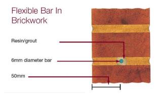
In general the reinforcement used is helical twisted stainless steel bar with diameters between 4mm and 8mm. Larger 10mm diameter bar is generally used for anchoring and tying.
